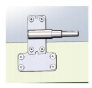
Step 13: Install the arm bracket plate at the appropriate location and install the arm bracket.
