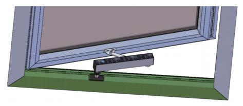
Step 10: When the window sill space is too small to place the mounting bracket, you can choose a side-mounted bracket to install on the side of the window sill.
