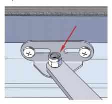
Step 8: Adjust the magnet position to adjust the window opening angle. The position of the magnet is the stopping position of the window opener.
