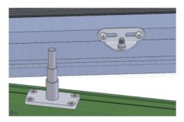
Step 3: The installation angle of the window opener should be slightly tilted outwards.
