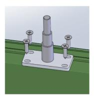
Step 2: Install the arm bracket on the window. When installing the arm bracket, the window opener should be installed on bracket 1 and close the window to confirm the position of the arm bracket.
