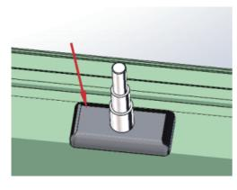
Step 5: Install the magnetic limit switch.
