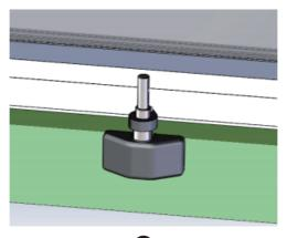
Step 12: When the window is an outward-opening type, it can be installed through an outward-opening bracket. Install the wider one on the side of the window sill and install the measuring bracket.
